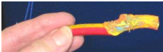
Joe's damaged electrical cord
