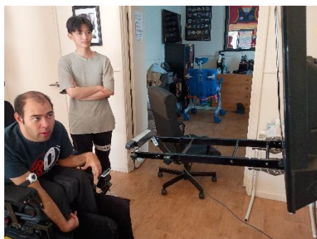
A custom made frame to support Edwards eye-gaze equipment
